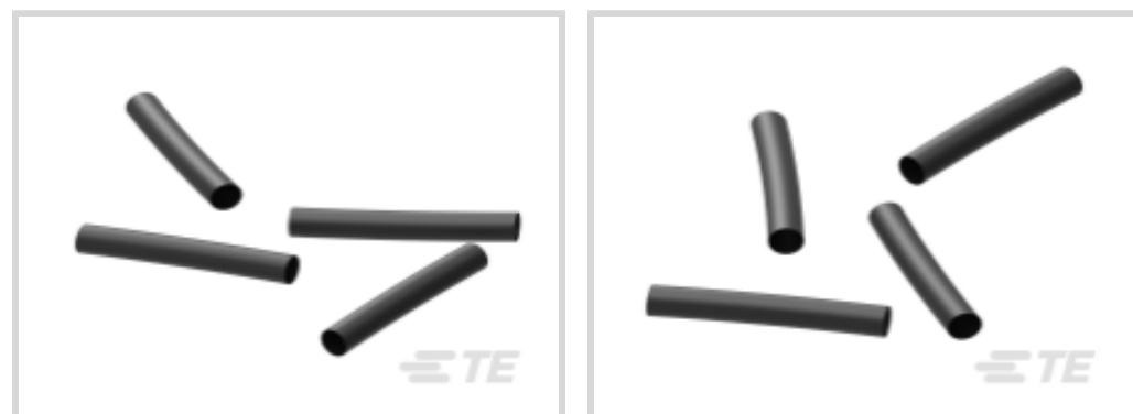
Tubing Product Type: **Heat Shrink Tubing**Primary Product Color: **Black**Shrink Ratio: **2:1**Wall Type: **Single Wall**Recovered Inside Diameter (Max): **3.18 mm [.125 in]**[All RW-175 Heat Shrink Tubing \(57\)](#)
